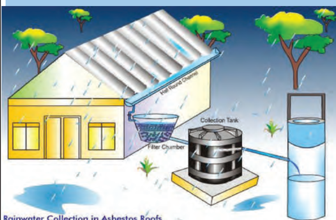
Rainwater Collection in Asbestos Roofs
